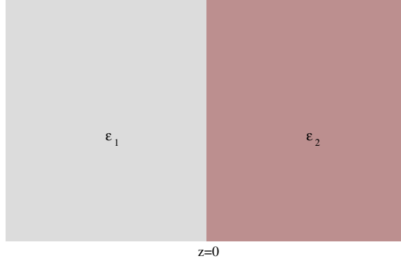
Figure 1. Two semi-infinite media with dielectric functions \epsilon_1 and \epsilon_2 separated by a planar interface at z = 0 .
