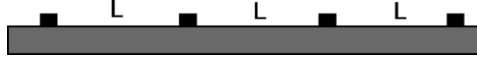
Figure 30. A periodic grating of constant L . The grating periodic structure can provide an impinging free electromagnetic radiation with additional momentum 2\pi/L .
