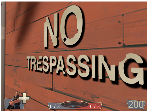
Figure 7: Soft drop-shadow added by the pixel shader. The direction, size, opacity, and color of the shadow are dynamically controllable.
