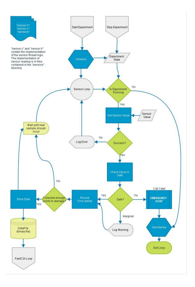
Figure 3.1: Flow chart for a sensor thread
