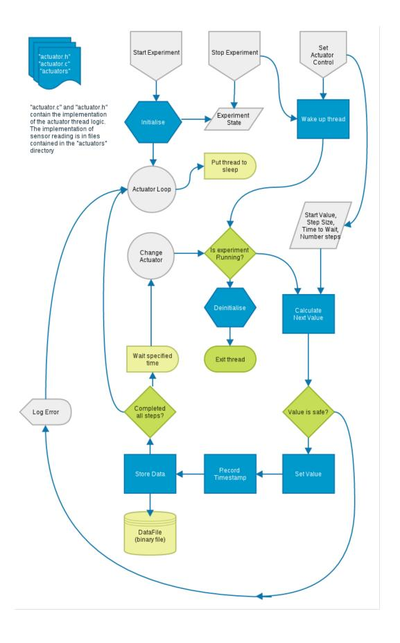
Figure 3.2: Flow chart for an actuator thread
