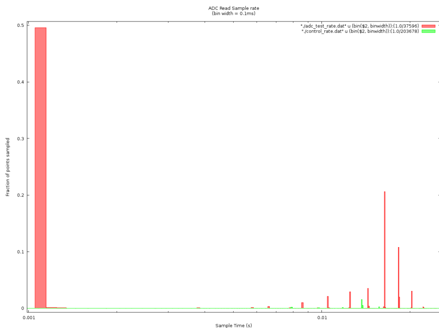
Figure 4: Same graph as Figure 2.3 but zoomed in to highlight the distribution obtained with ADC_Read is called.
