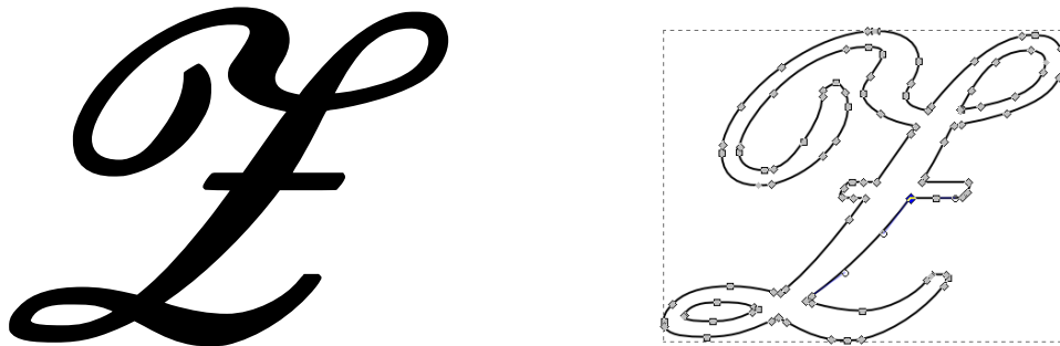
Figure 3.5: a) Vector glyph for the letter Z b) Screenshot showing Bézier control points in Inkscape
