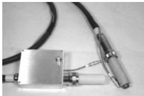
Grid pulsing cable for capacitive pulsing
