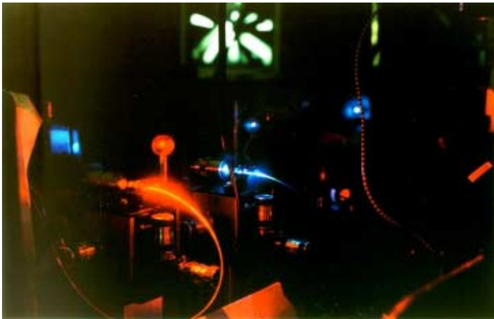
Fig. 5.3: Red and blue lasers coupled simultaneously into the SNOM fiber.
