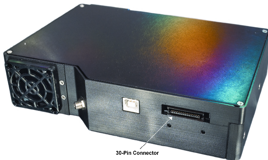
Location of QE65000 30-Pin Accessory Connector
