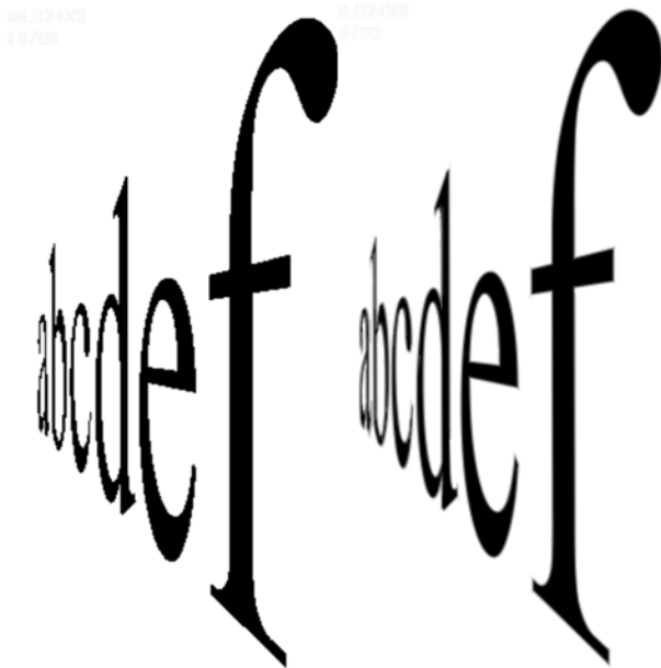
Figure 9: On the left is a vector image of text using just our in/out pixel shader. On the right is the result of our anti-aliasing scheme.
