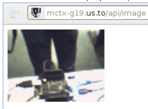
Figure 1: Image from Logitech webcam transferred through BeagleBone server
