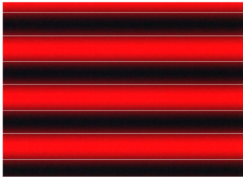
Figure 3: Image generated by interferometer test program. Nodes are identified with white lines.
