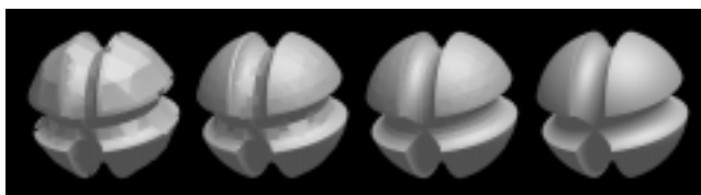
Figure 9. Four LOD models with varying amounts of error rendered from an ADF octree.
