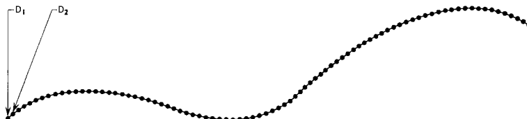
Figure 2 Curve defined by linear segments joining data points
