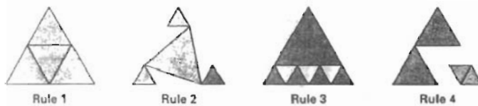
Figure 10-105 Four geometric substitution rules for subdividing and altering the shape of an equilateral triangle.
