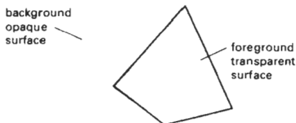
Figure 13-8 Viewing an opaque surface through a transparent surface requires multiple surface-intensity contributions for pixel positions.
