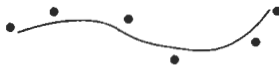
Figure 10-20 A set of six control points approximated with piecewise continuous polynomial sections
