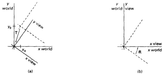
Figure 6-4 A viewing-coordinate frame is moved into coincidence with the world frame in two steps: (a) translate the viewing origin to the world origin, then (b) rotate to align the axes of the two systems.
