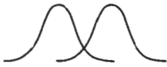
Figure 2-6 Two illuminated phosphor spots are distinguishable when their separation is greater than the diameter at which a spot intensity has fallen to 60 percent of maximum.
