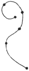
Figure 10-19 A set of six control points interpolated with piecewise continuous polynomial sections.
