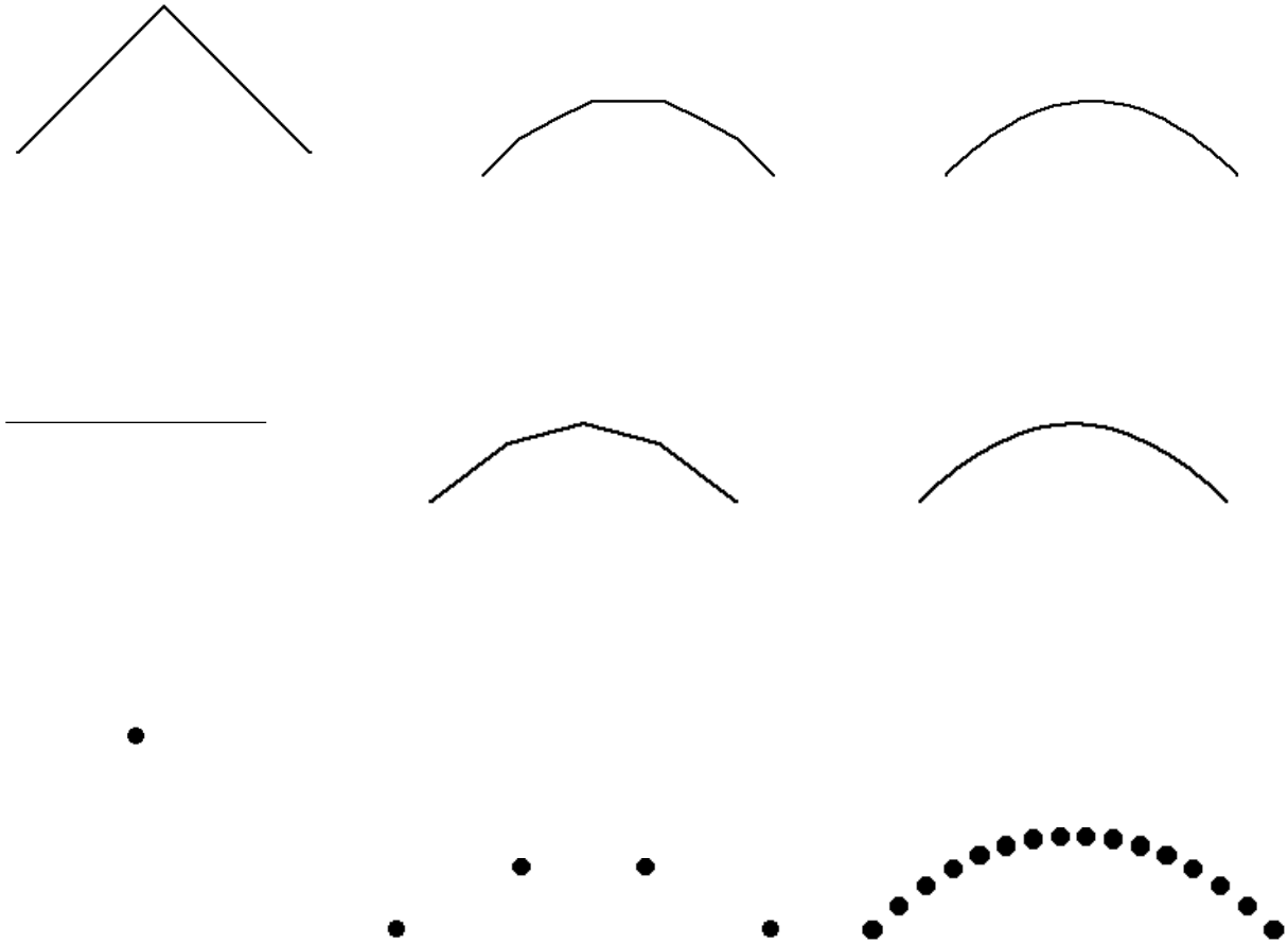
Figure 5: A quadratic Bezier curve generated from an iterated function system. The top row is generated in the usual manner starting from the control polygon; the middle row is generated starting from the chord joining the first and last control points instead of the control polygon; the bottom row is generated from a single point. In each case, levels 0, 2 and 4 of the iteration are illustrated.
