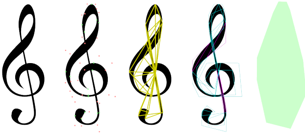
Figure 3: Filled path, with control points, with anchor geometry, and with cubic Bézier discard hulls, and conservative cover geometry.
