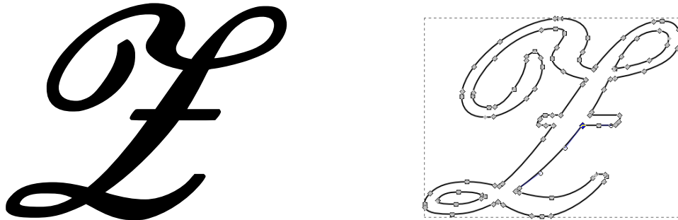
Figure 3.5: a) Vector glyph for the letter Z b) Screenshot showing Bézier control points in Inkscape
