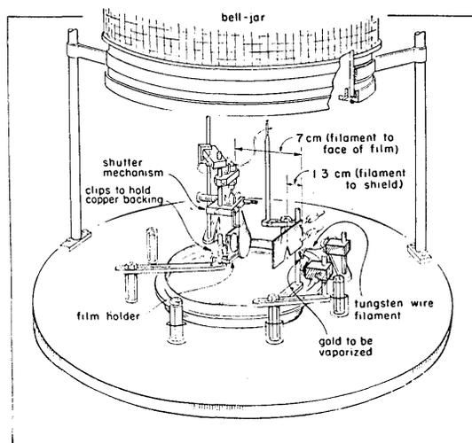
FIG. 1. Apparatus for the preparation of Gold Black.
