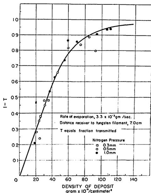
FIG. 2. Absorption of infra-red radiation by gold "blacks" as a function of density of deposit.
