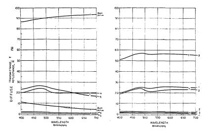
FIG. 4. Visible diffuse transmission and reflection of gold "blacks."
