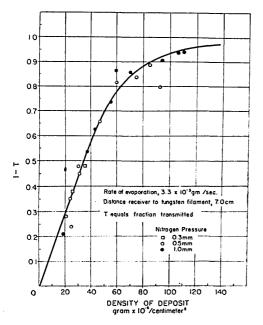
FIG. 2. Absorption of infra-red radiation by gold "blacks" as a function of density of deposit.
