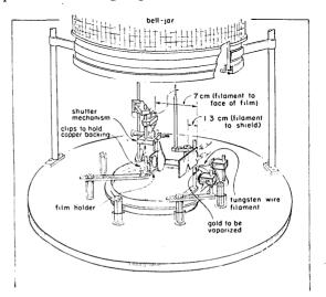
FIG. 1. Apparatus for the preparation of Gold Black.
